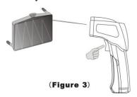
2. Locating a hot spot aim the thermometer outside the area of interest, then scan across with up and down motions until you locate the hot spot.(please turn on the laser to for accurate measuring)
