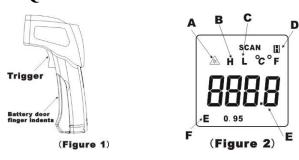
Press battery door clip, install battery correctly. Pull the trigger, LCD display reading & battery icon. Release the trigger and the reading will hold for 7 seconds
